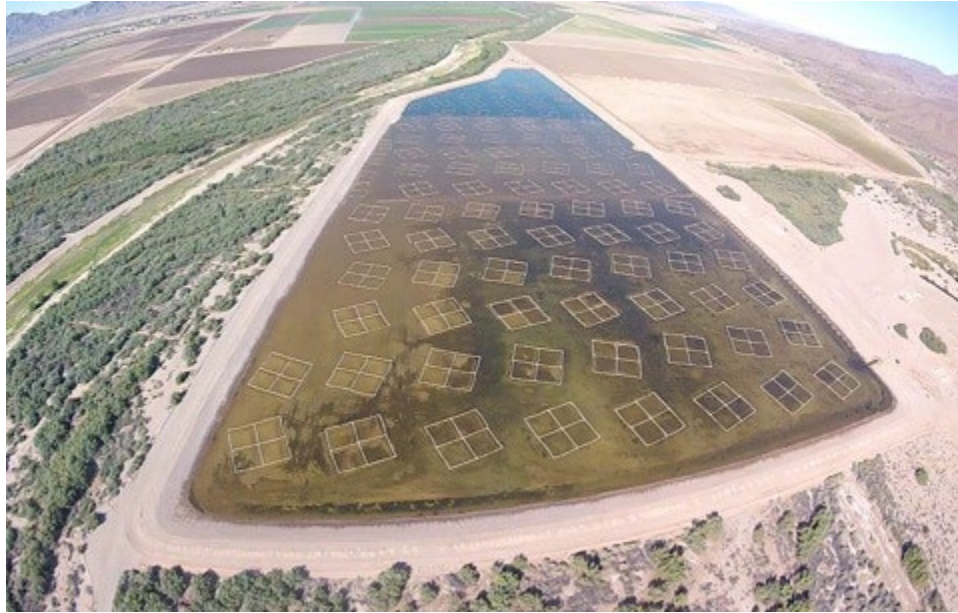
Figure 29. 60 acre Salinity Gradient Solar Pond constructed near Yuma, AZ
